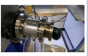
Measured in line viscosity with Soflux (at about 1 000 s<sup>-1</sup>) of 245 Pa.s, correlated to the lab measurement at 1 s<sup>-1</sup> of 10 208 Pa.s
